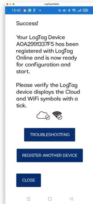
You can repeat this process at any time, however, the logger must not be recording, or you will receive an error message.
