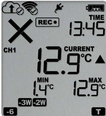
Each alarm trigger condition consists of a threshold temperature value, an activation type (which can be instant, consecutive or accumulative<sup>4</sup>) and a delay time, if it is not an instant alarm.
