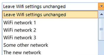
You can also type a new SSID directly if the wireless network for which the unit is set up is not available where you complete the configuration.
