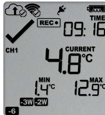
The logger has successfully completed its initial connection process.
