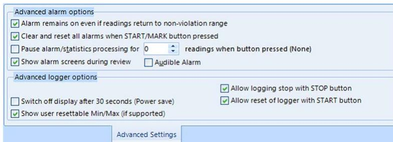
Figure 7: UTRED30-WiFi advanced configuration screen in LogTag<sup>®</sup> Analyzer 3
