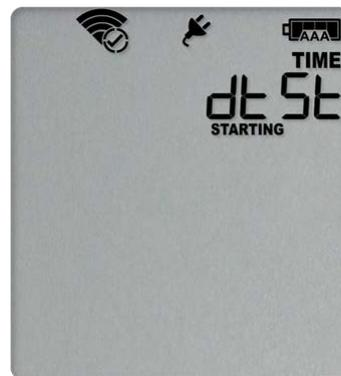
The UTRED30-WiFi will perform a [Connection Test](#) as soon as the recording has started. To check the connection before the start time is reached, you can initiate the connection test yourself. Please refer to [Testing your wireless and network connection \(on page 35\)](#).
