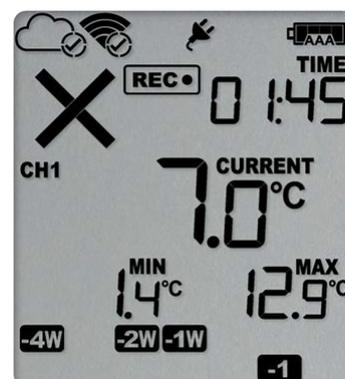
In this example the paused function was activated, and the paused symbol is shown on the display. For more information about paused readings please see the section about [Paused Readings on the next page](#).
