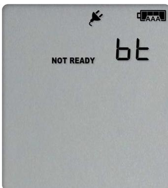
If the display does not show **bt**, you can activate the Bluetooth function by pressing and holding the **Channel/FUNCTION** button until **bt** appears.
