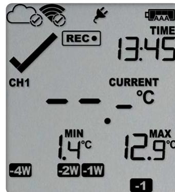
When evaluating data, any readings taken while the probe is disconnected are shown as **--.-** in the data list. The chart in LogTag<sup>®</sup> Analyzer and in LogTag<sup>®</sup> Online will show a gap during this period. Minimum and Maximum values shown on the display will remain visible and will not be updated until the sensor is plugged back in.
