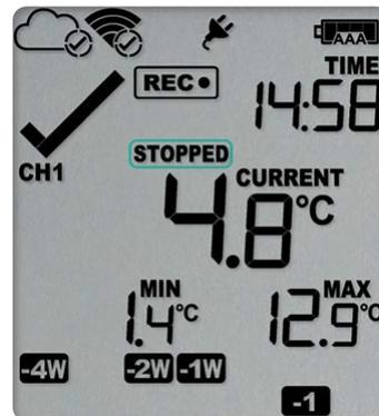
Keep holding the button until the **REC•** symbol disappears, then release the button within 2 seconds.
