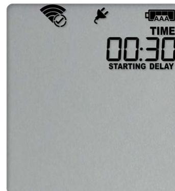
As with a regular push button start without delay, the UTRED30-WiFi will perform a [Connection Test](#) as soon as the recording has started. To check the connection before the delay value has elapsed, you can initiate the connection test yourself. Please refer to [Testing your wireless and network connection \(on page 35\)](#).
