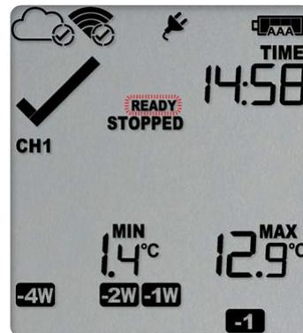
When the **STOPPED** symbol turns off, release the button within 2 seconds. The logger is now ready to be started again. Follow the normal starting procedure ([Starting the Logger on page 49](#)).
