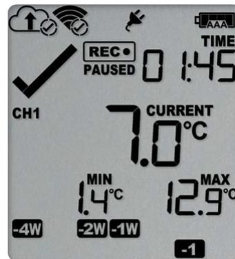
**⚠** Note: Only the Alarm Indicator (×) can be cleared! The day alarm marker (-1 in the above example) remains shown, as it is part of the statistic summary. Clearing an alarm also does not reset any of the delay values. Please see [Alarm Configuration](#) for additional information.
