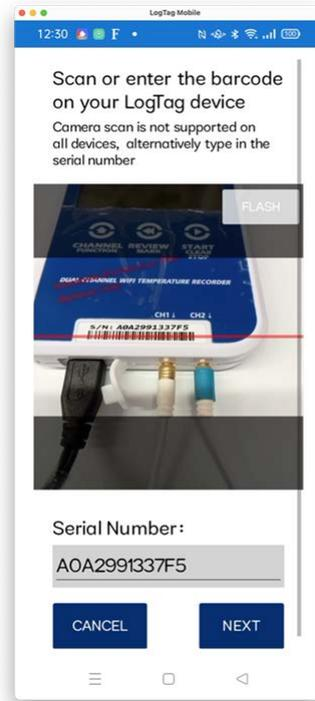
At this point, plug the power supply into the UTRED30-WiFi. When you connect a UTRED30-WiFi to power for the first time, the logger's Bluetooth function will be activated automatically, allowing your smart device to connect. No specific pairing action is required. The logger should show the following display:
