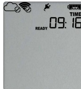
If the button is released while **STOPPED** is still on, or you wait until the **READY** symbol disappears, the display shows **STOPPED** again, and the logger remains stopped. This means, the data from the previous trip is still accessible.
